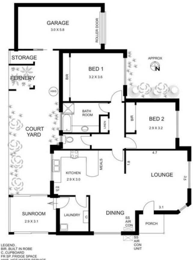
C..CUPBOARD FR SP. FRIDGE SPACE HWS..HOT WATER SERVICE SS AIR CON..SPLIT SYSTEM AIRCONDITIONER SS AIR CON UNIT. SPLIT SYSTEM AIRCONDITIONER UNIT
